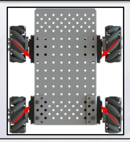
Put the mecanum wheels on your chassis. There are two types of wheels so when putting them on the chassis make sure the diagonal of the small wheels on the mecanum wheels point towards the center of the robot as shown.
