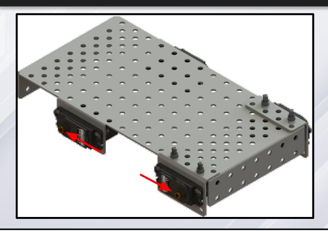
Repeat at all four positions on the brackets and chassis. Make sure the spline of the motor face away from the center of the chassis.
